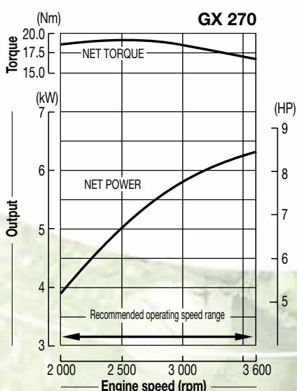
The power rating of the engine indicated in this document is the net power tested on a production engine for the engine model and measured in accordance with SAE J1349 at a specified rpm. Mass production engines may vary from this value. Actual power output for the engine installed in the final machine will vary depending on numerous factors, including the operating speed of the engine in application, environmental conditions, maintenance, and other variables.
