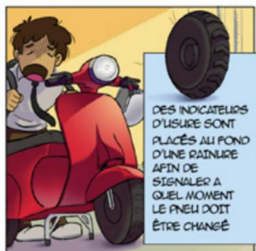
DES INDICATEURS D'USURE SONT PLACÉS AU FOND D'UNE RAINURE AFIN DE SIGNALER A QUEL MOMENT LE PNEU DOIT ÊTRE CHANGÉ
