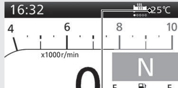
Air temperature gauge
