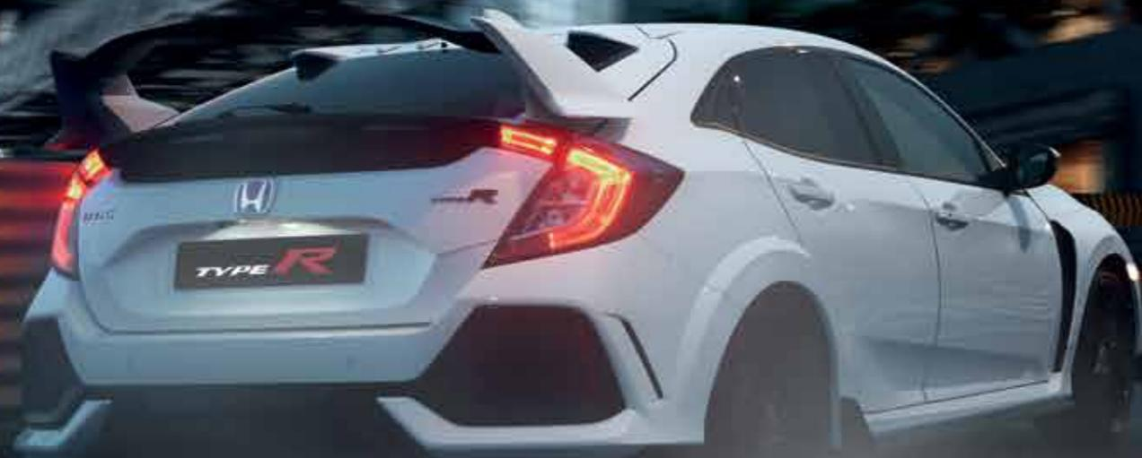
High performance technology requires unique, motorsport inspired features such as brake cooling vents, aerodynamic rear wing, lightweight aluminium vented bonnet and centre mounted triple outlet exhaust.
